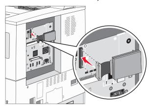
8 Press the three posts on the mounting plate into the holes on the system board. The hard disk *snaps* into place.
